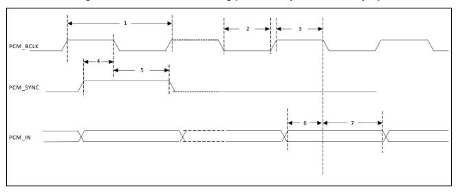
Table 9: PCM Burst Mode (Receive Only, Short Frame Sync)
