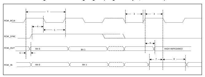
Table 8: PCM Interface Timing Specifications (Long Frame Sync, Slave Mode)
