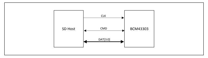
Figure 25: Signal Connections to SDIO Host (SD 1-Bit Mode)
