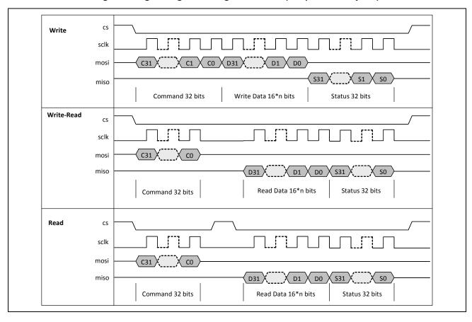
Figure 31: gSPI Signal Timing with Status (Response Delay = 0)
