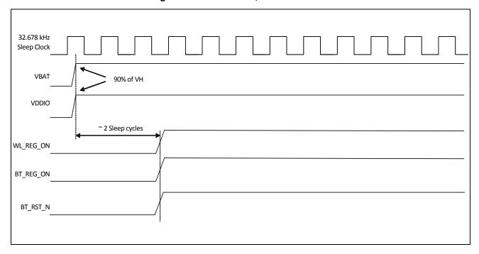
Figure 46: WLAN = OFF, Bluetooth = OFF
