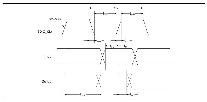
Figure 43: SDIO Bus Timing (High-Speed Mode)
