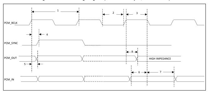
Table 5: PCM Interface Timing Specifications (Short Frame Sync, Master Mode)
