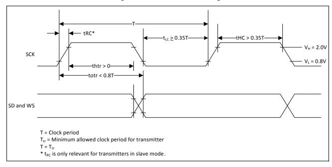
Figure 20: I<sup>2</sup>S Receiver Timing
