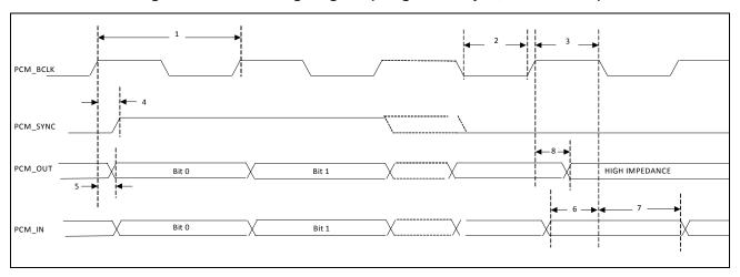
Table 7: PCM Interface Timing Specifications (Long Frame Sync, Master Mode)
