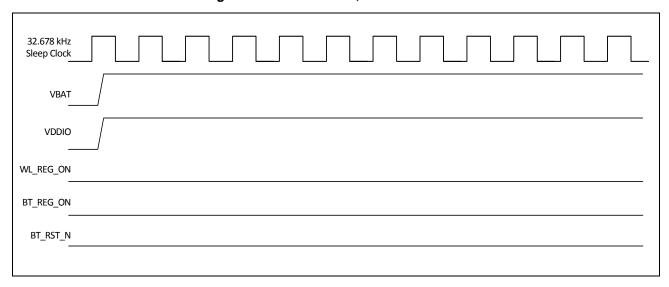
Figure 47: WLAN = ON, Bluetooth = OFF
