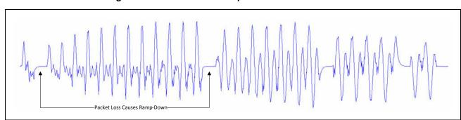
Figure 9: CVSD Decoder Output Waveform Without PLC
