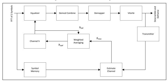
Figure 36: STBC Receive Block Diagram
