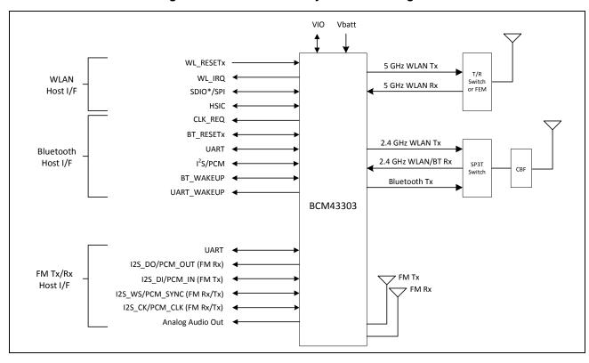
Figure 3: Mobile Platform System Block Diagram
