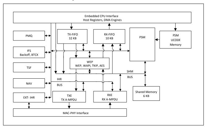
Figure 34: WLAN MAC Architecture
