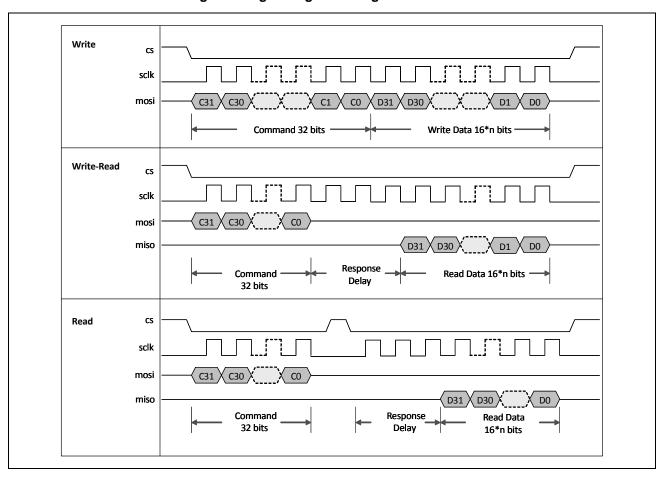
Figure 30: gSPI Signal Timing Without Status
