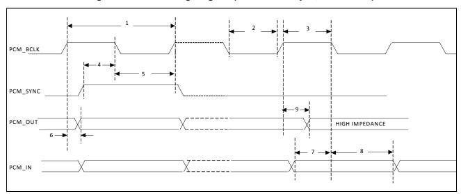
Table 6: PCM Interface Timing Specifications (Short Frame Sync, Slave Mode)
