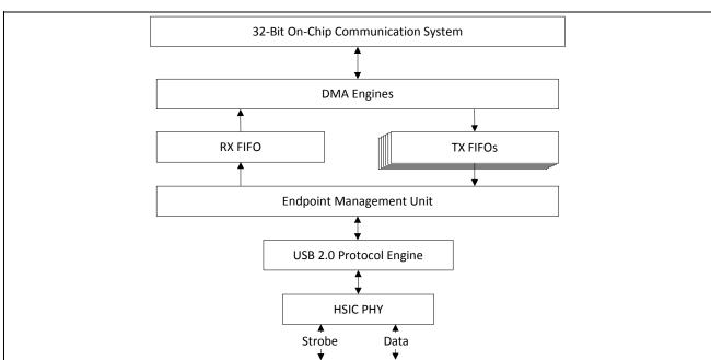
Figure 33: HSIC Device Block Diagram
