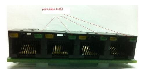
Figure 4: LEDs Indication
