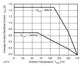
Fig. 1 - Forward Current Derating Curve
