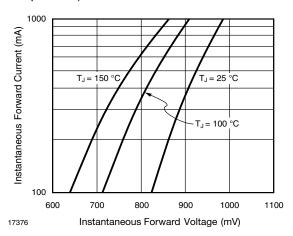
Fig. 2 - Typical Instantaneous Forward Characteristics
