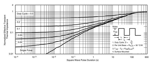
Normalized Thermal Transient Impedance, Junction-to-Ambient
