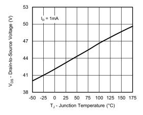
Drain Source Breakdown vs. Junction Temperature
