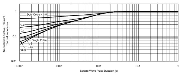
Normalized Thermal Transient Impedance, Junction-to-Case
