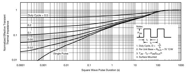
Normalized Thermal Transient Impedance, Junction-to-Ambient
