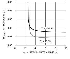
On-Resistance vs. Gate-to Source Voltage
