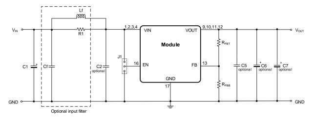
The 171011801 integrates both the input and output capacitors. Therefore, additional external input/output capacitors are normally not required.
