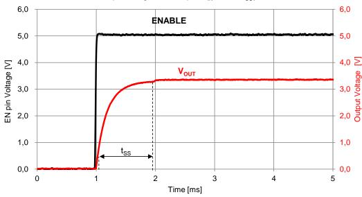
Output Voltage at Start Up -  $V_{IN} = 12V$ ,  $V_{OUT} = 3.3V$
