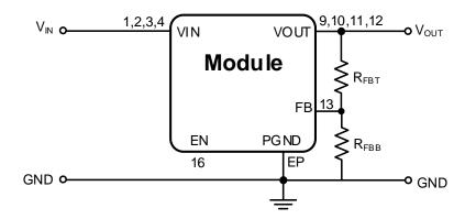
The only external components necessary to operate the 171011801 that must be placed on the PCB are the resistors of the output voltage divider, as shown in the picture above.
