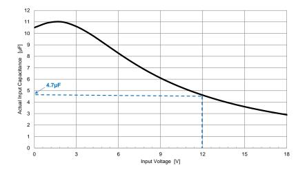
From the diagram above, the actual capacitance value of  $4.7\mu$ F can be read.
