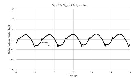
In case the application has more demanding requirements in terms of output voltage ripple, additional external capacitors should be used. The value of the external additional capacitance ( $C_{OUT,INT}$ ) can be calculated using the following equation:
