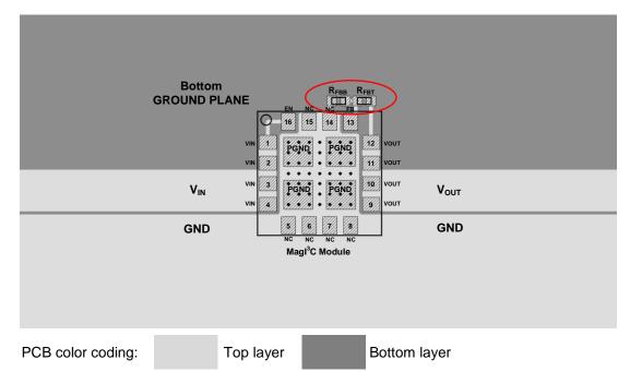
The resistor divider ( $R_{FBT}$  and  $R_{FBB}$ ) should be located close to the FB pin. Since the FB node is high impedance, the trace thickness should be kept small. The traces from the FB pin to the middle point of the resistor divider should be as short as possible. The upper terminal of the output resistor divider (where the V<sub>OUT</sub> is applied) should have a short connection to the VOUT pins, where internally are integrated the output capacitors.
