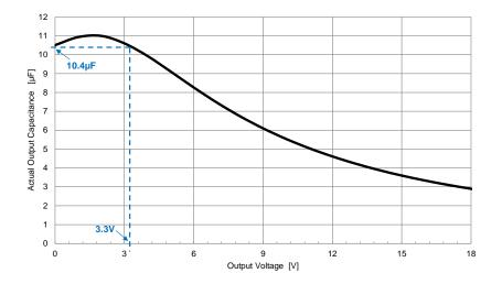
At  $V_{OUT}$  = 3.3V the value of the output capacitance is not reduced due to the voltage, it is instead slightly higher. Nevertheless, a total value of 20µF can be considered for C<sub>OUT, INT</sub>.
