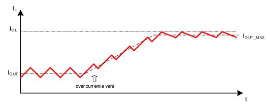
During overcurrent condition, the duty cycle is no longer determined by the control loop, it is instead limited by the current limit threshold. Therefore, the output voltage is out of regulation and drops (see figure below).
