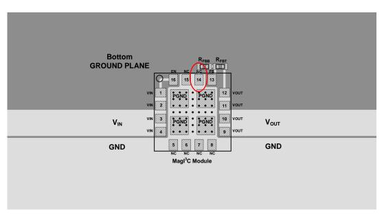
The ground connection of the lower resistor of the output voltage divider ( $R_{FBB}$ ) should be routed to the PGND pins of the device. If not properly handled, poor grounding can result in degraded load regulation or erratic output voltage ripple behavior.
