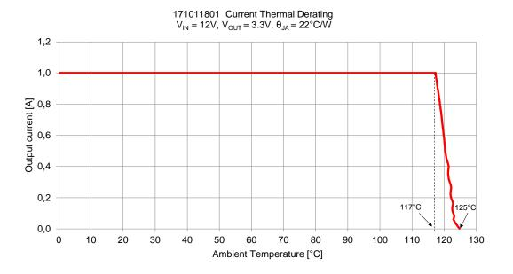
The ambient temperature and the power limits of the derating curve represent the operation at the max junction temperature specified in the "Operating Conditions" section on page 4.
