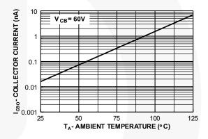
Figure 6. Collector Cut-Off Current vs.
