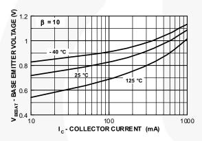
Figure 5. Base-Emitter Saturation Voltage vs.
