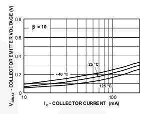
Figure 4. Collector-Emitter Saturation Voltage vs.
