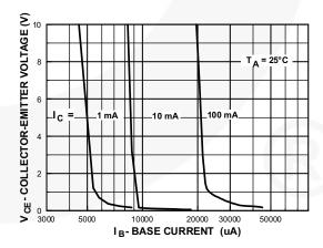
Figure 8. Collector Saturation Region
