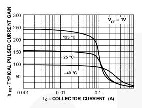
Figure 3. Typical Pulsed Current Gain vs.
