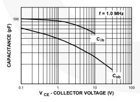
Figure 7. Input and Output Capacitance vs. Reverse Voltage
