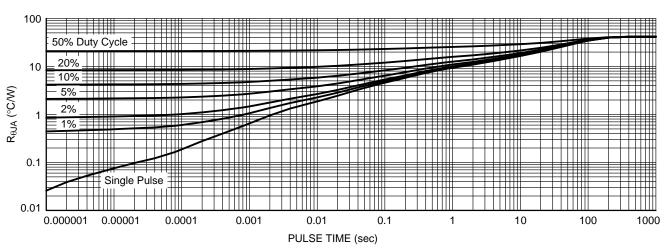
Figure 13. Thermal Characteristics
