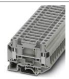
Feed-through terminal block, Connection method: Screw connection, Cross section: 0.5 mm² -10 mm², AWG: 20 - 10, Width: 8.2 mm, Mounting type: NS 35/7,5, NS 35/15, NS 32, Color: gray
