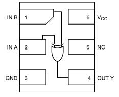
Figure 1. Pinout (Top View)
