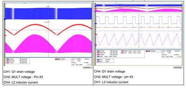
In *Figure 13* and *15* the detail of the waveforms at switching frequency allows measuring the operating frequency and the current peak at top of the input sine wave during operation at 100 Vac and 230 Vac. The multiplier waveform has been captured as a reference.
