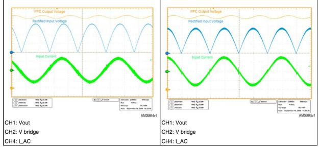
The power factor (PF) and the total harmonic distortion (THD) have been measured too and the results are shown in *Figure 7* and *8*. As visible, the PF remains close to unity throughout the input voltage mains and the total harmonic distortion is very low.
