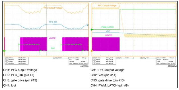
The event of an open loop is captured in *Figure 30*. We can notice the protection intervention, latching the operation of the L6563S. As mentioned previously, to restart the system the input power must be recycled.
