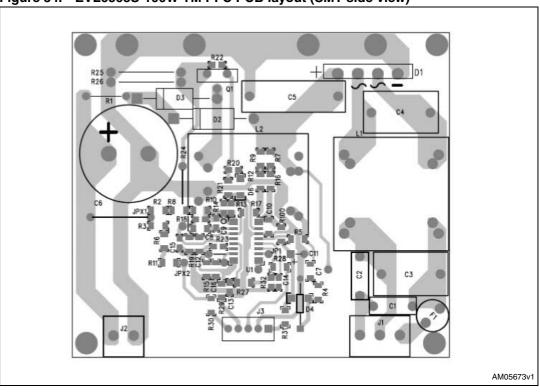
Figure 34. EVL6563S-100W TM PFC PCB layout (SMT side view)
