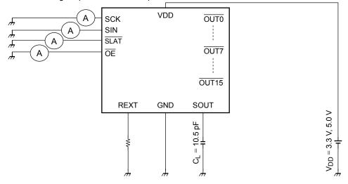
Test Circuit4: Power supply current
