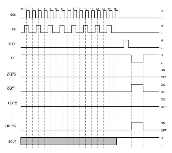
• The latch circuit is a leveled-latch circuit. Please exercise precaution as it is not triggered-latch circuit.
