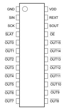
Short circuiting an output pin to a power supply pin (Power-supply voltage  $V_{DD}$  and LED anode power supply), or short-circuiting the REXT pin to the GND pin will likely exceed the absolute maximum rating, which in turn may result in smoldering and/or permanent damage. Please keep this in mind when determining the wiring layout for the power supply and GND pins.
