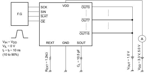
Test Circuit5: Constant current output / Output OFF leak current / Constant current error Constant current output power supply voltage regulation Constant current output output voltage regulation
