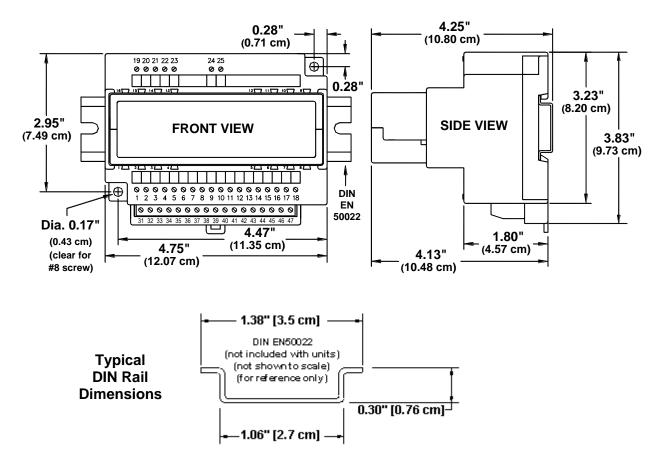
Figure 2-2 - VersaTRAK IPm2m RTU Dimensions
