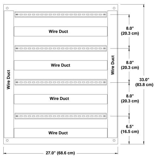
Figure 2-1 Sample Layout for a 36" x 30" Enclosure
