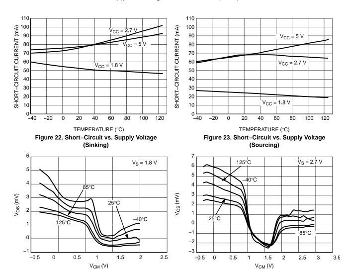
Figure 24. Offset Voltage vs. Common Mode Range V<sub>DD</sub> 1.8 V
