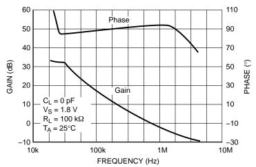
Figure 9. Gain and Phase vs. Frequency
