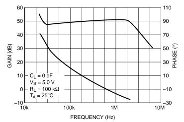
Figure 10. Gain and Phase vs. Frequency
