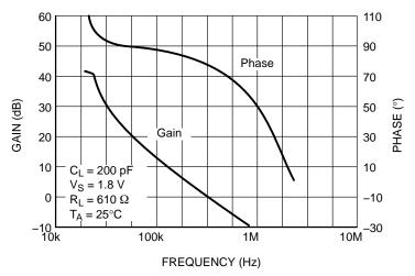
Figure 7. Gain and Phase vs. Frequency
