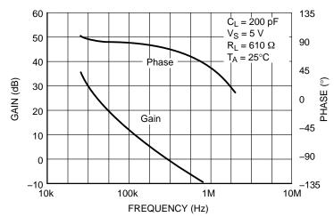
Figure 8. Gain and Phase vs. Frequency
