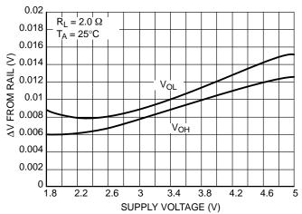
Figure 6. Output Voltage vs. Supply Voltage
