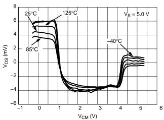
Figure 26. Offset Voltage vs. Common Mode Range V<sub>DD</sub> 5.0 V
