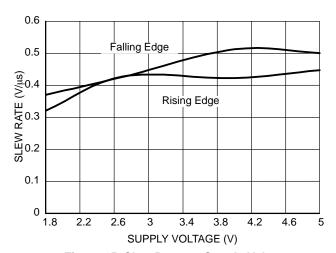
Figure 15. Slew Rate vs. Supply Voltage
