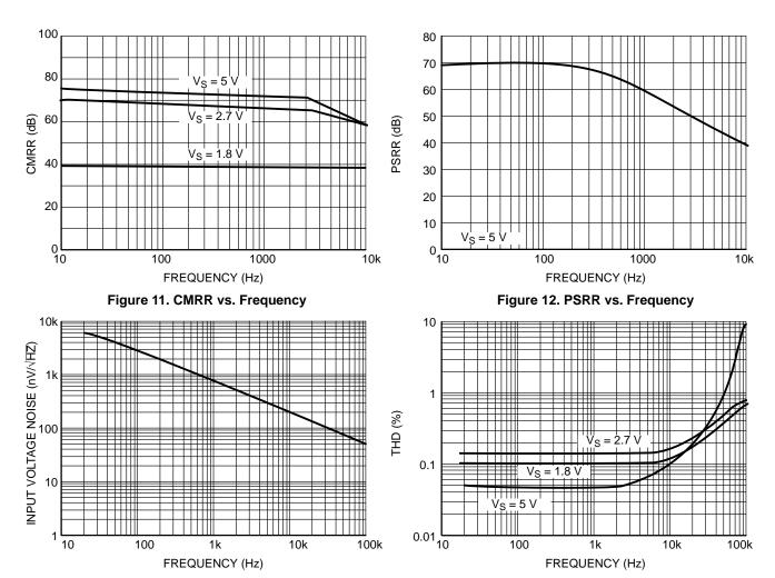
Figure 13. Input Voltage Noise vs. Frequency
