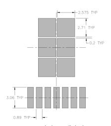
recommended stencil design solder paste recommendation 150μm
