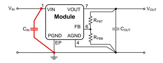
Based on those considerations, the path of the input capacitor  $C_{IN}$  is the most critical one to generate high frequency noise on Vin. Therefore place  $C_{IN}$  as close as possible to the Magl³C power module  $V_{IN}$  and PGND exposed pad EP. This will minimize the high di/dt area and reduce radiated EMI. Additionally, grounding for both the input and output capacitor should consist of a localized top side plane that connects to the PGND exposed pad.
