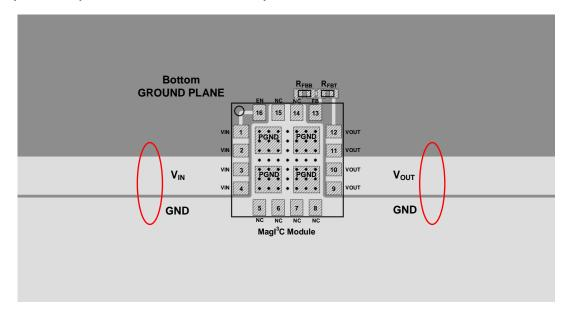
This reduces any voltage drops on the input or output of the converter and maximizes efficiency.
