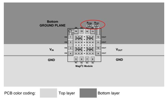
The resistor divider (R<sub>FBT</sub> and R<sub>FBB</sub>) should be located close to the FB pin. Since the FB node is high impedance, the trace thickness should be kept small. The traces from the FB pin to the middle point of the resistor divider should be as short as possible. The upper terminal of the output resistor divider (where the V<sub>OUT</sub> is applied) should have a short connection to the VOUT pins, where internally are integrated the output capacitors.
