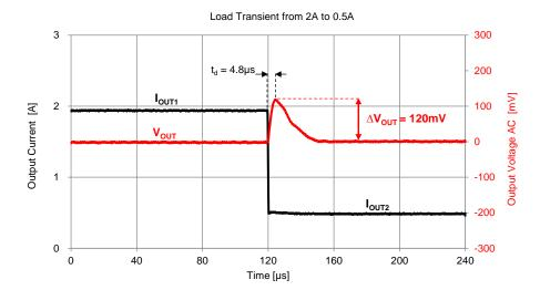
If the application demands a lower undershoot or overshoot, an additional external capacitance is necessary. In order to choose the value of the external output capacitor C<sub>OUT,EXT</sub>, the following steps should be utilized:
