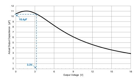
At  $V_{OUT} = 3.3V$  the value of the output capacitance is not reduced due to the voltage, it is instead slightly higher. Nevertheless, a total value of  $20\mu F$  can be considered for  $C_{OUT, INT}$ .
