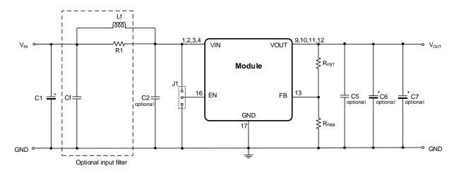
The 171021801 integrates both the input and output capacitors. Therefore, additional external input/output capacitors are normally not required.
