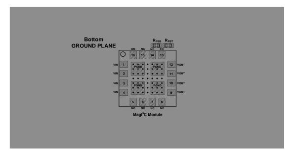
Place a dedicated solid ground copper area beneath the Magl<sup>3</sup>C Power Module.
