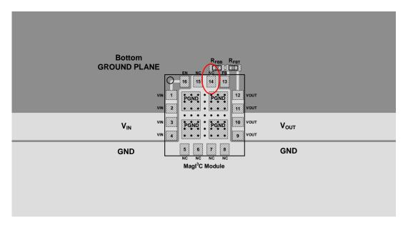
The ground connection of the lower resistor of the output voltage divider (R<sub>FBB</sub>) should be routed to the PGND pins of the device. If not properly handled, poor grounding can result in degraded load regulation or erratic output voltage ripple behavior.
