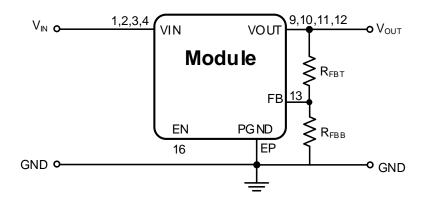
The only external components necessary to operate the 171021801 that must be placed on the PCB are the resistors of the output voltage divider, as shown in the picture above.
