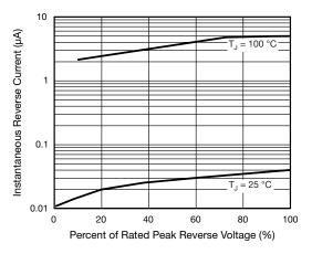
Fig. 4 - Typical Reverse Characteristics
