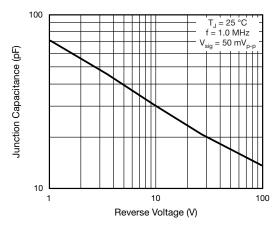
Fig. 5 - Typical Junction Capacitance
