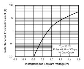
Fig. 3 - Typical Instantaneous Forward Characteristics
