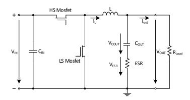
None of the required output capacitors are integrated within the module. A general recommendation in order to guarantee a stable behavior is to place at least a capacitance of 10µF (MLCC recommended) at the output.
