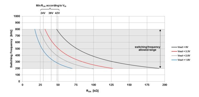
As stated above, the off-time is also limited to a minimum value of 260 ns, which limits the maximum duty cycle. Larger  $R_{\text{ON}}$  (lower  $F_{\text{SW}}$ ) should be selected in any application requiring large duty ratio.
