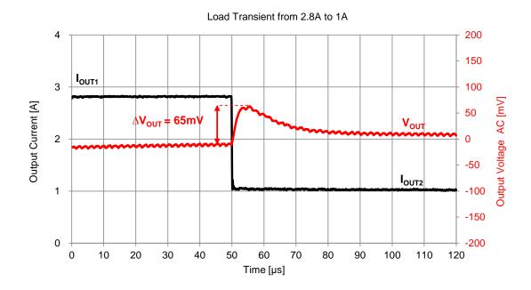
In both the positive and the negative transition, the  $\Delta V_{OUT}$  is significantly below the target (100mV). The explanation of the strong reduction of the  $\Delta V_{OUT}$  lies in the use of a capacitance value higher than the one calculated.
