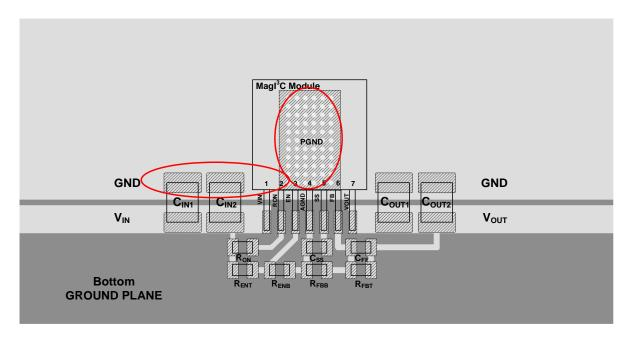
The negative terminal of  $C_{\text{IN1}}$  and  $C_{\text{IN2}}$  needs to be very close to the PGND pad of the power module.
