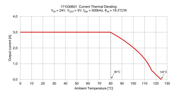
The ambient temperature and the power limits of the derating curve represent the operation at the max junction temperature specified in the "Operating Conditions" section on page 4.
