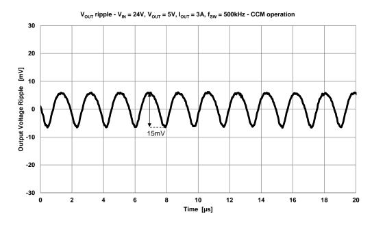
The output voltage ripple during CCM operation is much lower ( $<15mV_{pp}$ ) than the ripple during DCM operation (around  $35mV_{pp}$ ).
