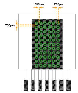
For best result, use a thermal via array as proposed in the picture above with drill of max 250µm, spaced 750µm apart. Ensure enough copper area is used for heat-sinking, to keep the junction temperature below 125°C.
