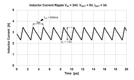
The load current where the transition between DCM and CCM takes place can be estimated using the following formula:
