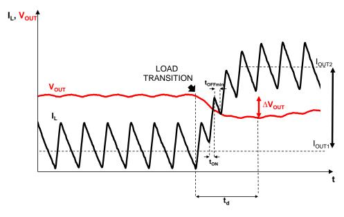
The selection of the  $C_{\text{OUT}}$  is related to the  $t_d$  as well as to the current step  $\Delta I_{\text{OUT}}$  and the max allowed voltage drop  $\Delta V_{\text{OUT}}$ , as shown by the following equation:
