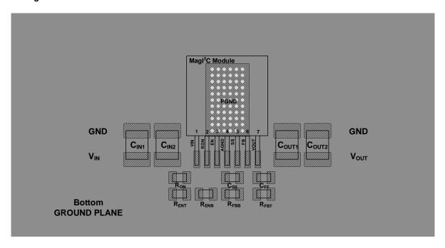
Place a dedicated solid GND copper area beneath the Magl<sup>3</sup>C Power Module.
