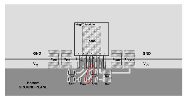
The ground connections for the soft-start capacitor (C<sub>SS</sub>), the output voltage lower resistor divider (R<sub>FBB</sub>) and enable components (when used) should be routed to the AGND pin of the device. If not properly handled, poor grounding can result in degraded load regulation or erratic output voltage ripple behavior. Place C<sub>SS</sub>, R<sub>FBT</sub> and R<sub>FBB</sub> close to their respective pins.
