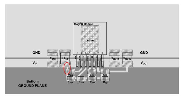
In order to avoid noise injection into RON pin, the resistor RoN should be routed to one of the input capacitors.
