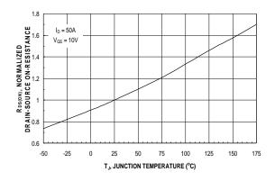
Figure 3. On-Resistance Variation with Temperature
