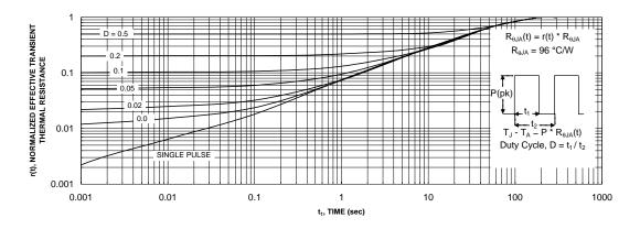
Figure 11. Transient Thermal Response Curve
