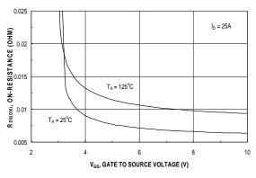
Figure 4. On-Resistance Variation with Gate-to-Source Voltage
