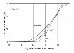
Figure 5. Transfer Characteristics
