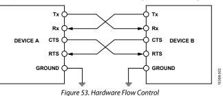
The flow control is bidirectional, meaning that both devices can request a halt in transmission. If one of the devices never requests a stop in transmission (for example, if the device is fast enough to always receive data), the CTS signal on the other device can be tied to the asserted logic level. Thus, the RTS pin on the fast device can become free to perform other functions.
