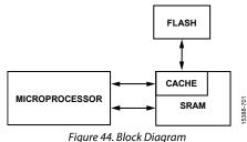
The ADuCM3027/ADuCM3029 cache architecture consists of a digital cache controller, a cache memory implemented as part of the system SRAM, a digital flash controller, and a flash memory. The cache architecture decreases the average latency of instruction and data accesses by utilizing the faster SRAM memory, and decreases the frequency of accesses to the relatively higher power flash memory.
