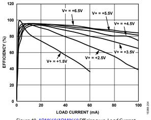
Figure 49. ADM660/ADM8660 Efficiency vs. Load Current
