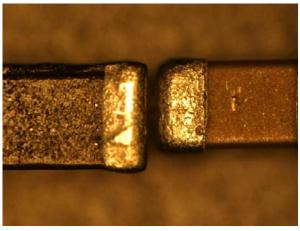
Figure 51. Width Comparison of a 0.1  $\mu F$  Capacitor (Right) vs. a 2.2  $\mu H$  Inductor (Left)
