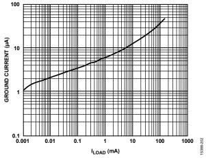
Figure 47. ADP165/ADP166 Ground Current vs. Load Current (ILOAD)
