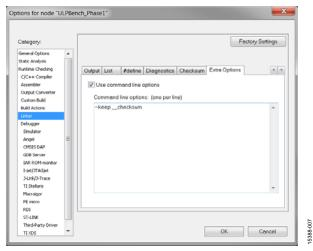
Figure 8. Linker > Extra Options Configuration Tab
