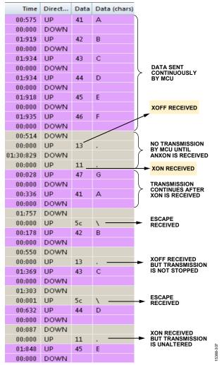
Figure 58. Data Capture Using a Sniffer Program
