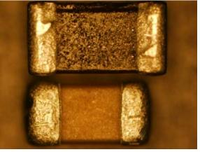
Figure 50. Length Comparison of a 0.1  $\mu$ F Capacitor (Bottom) vs. a 2.2  $\mu$ H Inductor (Top)
