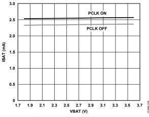
Figure 31. Impact of Peripheral Clock Gating on Active Mode Power Consumption
