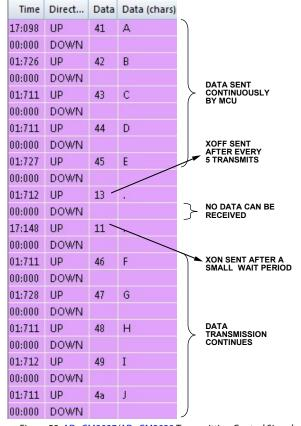
Figure 59. ADuCM3027/ADuCM3029 Transmitting Control Signals
