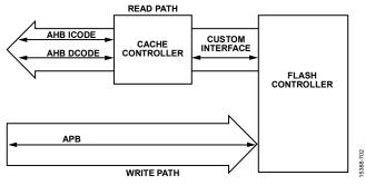
Figure 45. Flash and Cache Controllers
