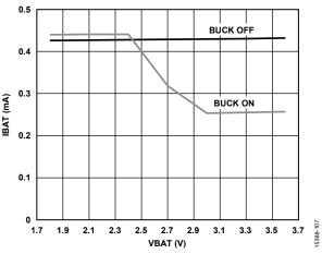
Figure 33. Impact of the Buck Converter on Flexi Mode Power Consumption
