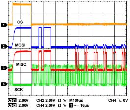
Figure 66. Page Read Start Sequence (Command and Address Bytes)
