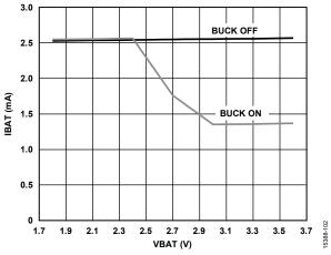
Figure 28. Impact of the Buck Converter on Active Mode Power Consumption Enabling Cache Memory
