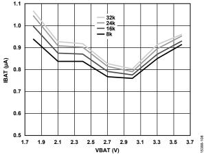
Figure 34. Current on the VBAT Supply Pin ( $I_{BAT}$ ) for Various Retained SRAM Values
