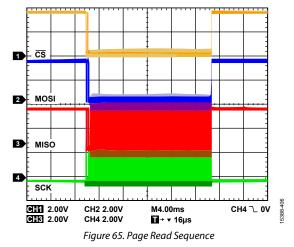
Figure 66 shows the start of the page read sequence where the ADuCM3027/ADuCM3029 transfers the command and address bytes. This transfer is followed by the page data from the serial flash memory.
