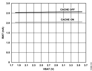
Figure 29. Impact of Cache Memory on Active Mode Power Consumption
