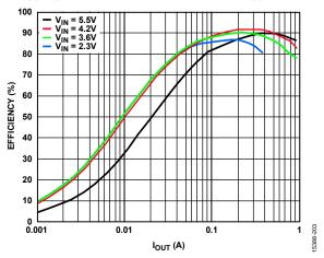
Figure 48. ADP2503/ADP2504 Efficiency vs. Output Current (IOUT)
