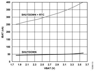
Figure 36. Shutdown Mode Current (External Sources vs. RTC0)
