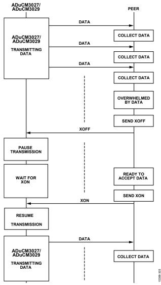
Figure 54. Software Flow Control Sequence Diagram
