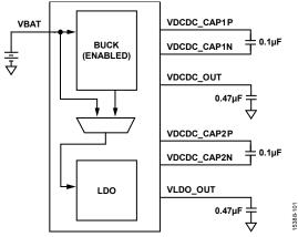
Figure 27. External Circuitry for Buck Converter Enabled Designs
