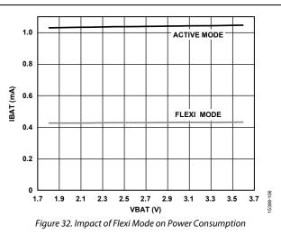
As shown in Figure 32, there is nearly a 66% savings in power when Flexi mode is used while the DMA is ongoing, rather than keeping the core in active mode.
