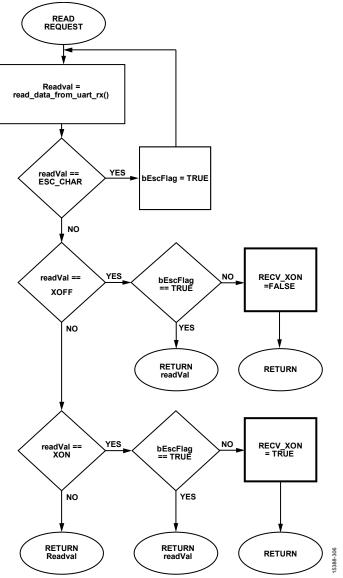
Figure 57. Flowchart of the Control Signals in the ISR Being Processed
