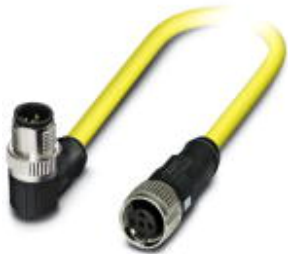
Sensor/Actuator cable, 5-position, PVC, yellow, Plug angled M12 SPEEDCON, A-coded, on Socket straight M12 SPEEDCON, A-coded, Cable length: 0.5 m
