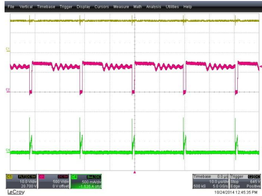
Figure 14. 460 V AC , Full-Load Condition (CH1: V CC (10 V/div), CH2: V DS (500 V/div), CH4: I DS (500 mA/div), Time: 10 μs/div)
