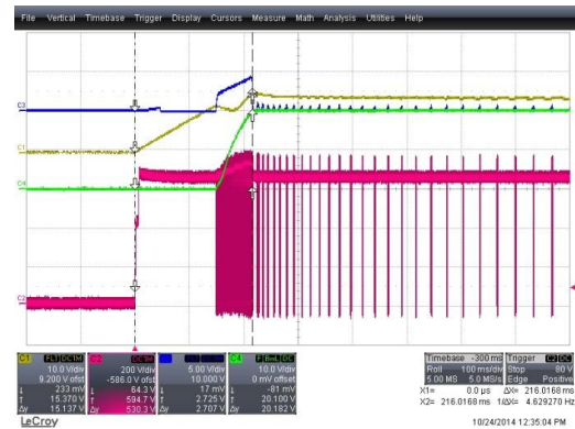
Figure 12. Startup Time = 216 ms, 460 V AC , Full-Load Condition (CH1: V CC (10 V/div), CH2: V DS (200 V/div), CH3: V FB (5 V/div), CH4: V OUT (10 V/div), Time: 100 ms/div)
