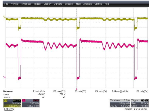
Figure 18. V_{DS}=786\text{ V} , V_{DIODE}=249\text{ V} , Steady-State, Full-Load Condition, 460\text{ V}_{AC} , (CH1: V_{DIODE} (200 V/div), CH2: V_{DS} (200 V/div), Time: 5 µs/div)
