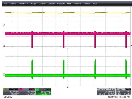
Figure 16. 460 V AC , No-Load Condition (CH1: V CC (10 V/div), CH2: V DS (500 V/div), CH4: I DS (500 mA/div), Time: 20 ms/div)
