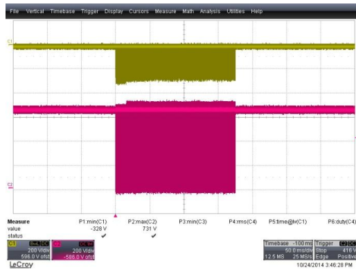
Figure 19. V_{DS}=731\text{ V} , V_{DIODE}=328\text{ V} , Output Short, Full-Load Condition, 460\text{ V}_{AC} , (CH1: V_{DIODE} (200 V/div), CH2: V_{DS} (200 V/div), Time: 50 ms/div)
