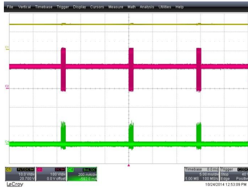
Figure 15. 85 V AC , No-Load Condition (CH1: V CC (10 V/div), CH2: V DS (100 V/div), CH4: I DS (200 mA/div), Time: 5 ms/div)
