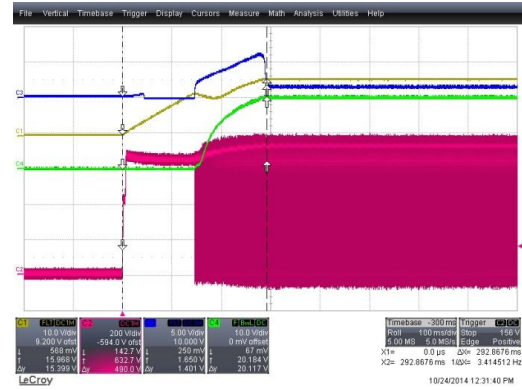
Figure 10. Startup Time = 293 ms, 460 V AC , Full-Load Condition (CH1: V CC (10 V/div), CH2: V DS (200 V/div), CH3: V FB (5 V/div), CH4: V OUT (10 V/div), Time: 100 ms/div)
