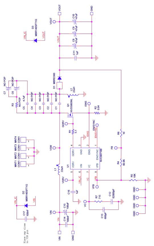
Figure 5. NCV887100 SEPIC Evaluation Board Schematic
