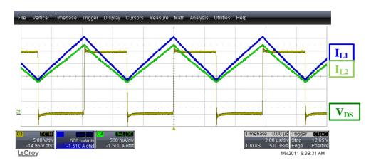
Figure 4. Operational Waveforms, V\_IN = 12 V, R\_{OUT} = 6  $\Omega$
