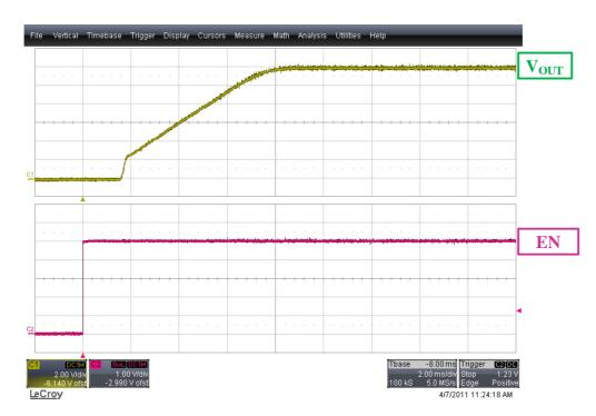
Figure 3. Typical Start–up with V $_{\text{IN}}$  = 12 V, R $_{\text{OUT}}$  = 6  $\Omega$
