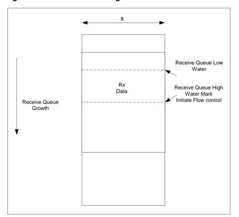
Figure 8-5. Flow Control Using Pause Control Frame
