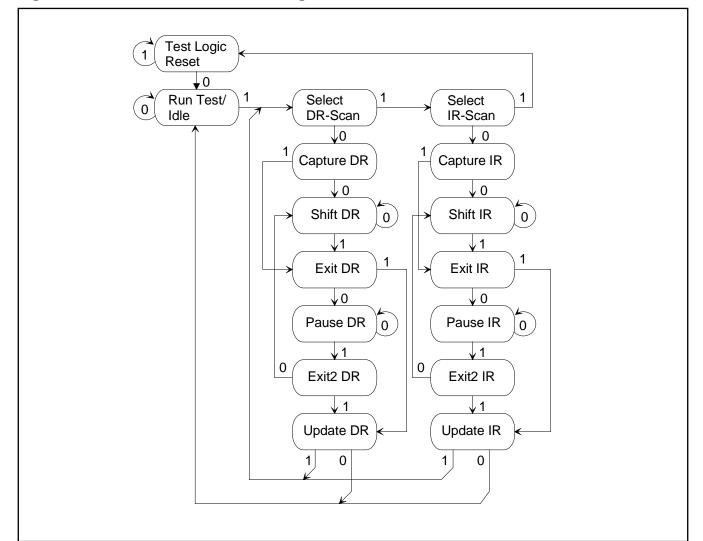
Figure 12-2. TAP Controller State Diagram
