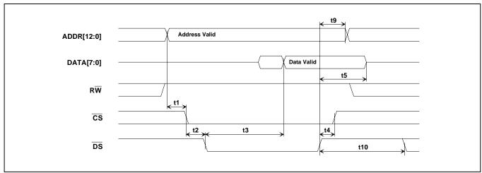
Figure 11-11. Motorola Bus Read Timing (HWMODE = 0, MODEC = 01)
