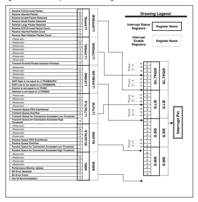
Figure 8-2. Device Interrupt Information Flow Diagram
