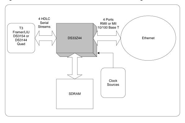
Figure 3-4. Ethernet Over DSL
