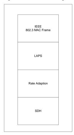
Figure 8-14. X.86 Encapsulation of the MAC Field
