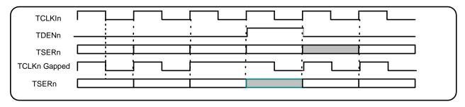
Figure 10-2. Rx Serial Interface Functional Timing
