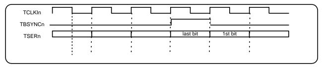
Figure 10-4. Receive Byte Sync Functional Timing
