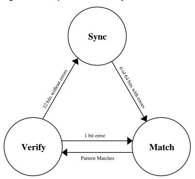
Figure 8-12. Repetitive Pattern Synchronization State Diagram
