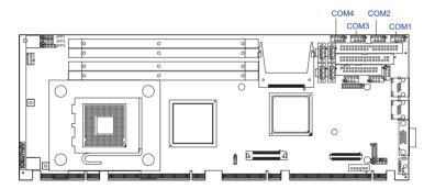
The PCE-5120 offers four serial ports COM1, COM2, COM3 and COM4. These ports can connect to serial devices, such as a mouse or to a communications network. The COM2 port can be configured to support RS-232/422/485 by pin header (JSETCOM2) setting, please refer to 1.8.4 for the information.
