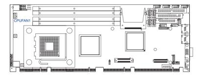
If a fan is used, this connector supports cooling fans of  $12V/1A\ (12W)$  or less.
