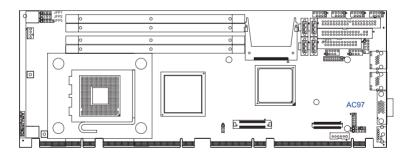
The PCE-5120 provides AC'97 audio through PCA-AUDIO-00A1 module from Advantech
