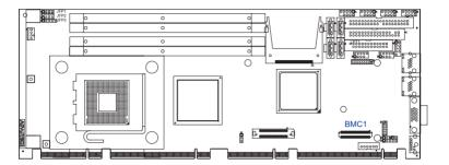
PCE-5120 is designed for supporting IPMI 2.0. The BMC module is mounted on board through this connector. For more detail operating information, please refer to Chapter 9.
