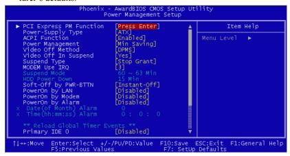
Figure 3.9: Power management setup screen (1)
