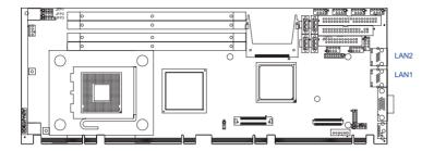
PCE-5120 uses the Intel 82573V Gigabit LAN chip which is linked to PCIe x1 Link. With this chip PCE-5120 may provide high throughputs for heavy loading networking environment. It provides two or one RJ-45 connectors in the rear side and is convenient for most industrial applications.
