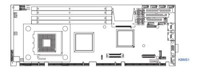
One 6-pin mini-DIN connectors (KBMS1) on the card mounting bracket provide connection to a PS/2 keyboard or a PS/2 mouse, respectively. KBMS1 can also be connected to an adapter cable (P/N: 1700060202) for connecting to both a PS/2 keyboard and a PS/2 mouse.
