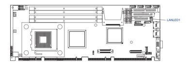
PCE-5120 provides an external LAN LED Pin header for connecting to the front side of the chassis. With this convenient design users may know whether the LAN port is acting or not easily. Refer to Appendix B for detailed information on the pin assignments.
