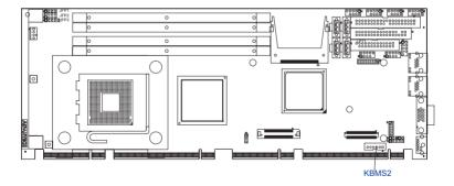
In addition to the PS/2 mouse/keyboard connector on the PCE-5120's rear plate, there is also an extra onboard external keyboard and mouse connector. This gives system integrators greater flexibility in designing their systems.
