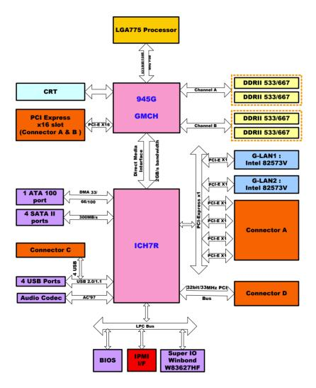
Figure 1.2: PCE-5120 Block Diagram
