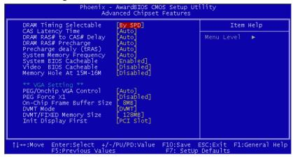
Figure 3.4: Advanced chipset features screen
