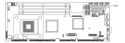
You can attach up to two IDE (Integrated Drive Electronics) drives to the PCE-5120's built-in controller
