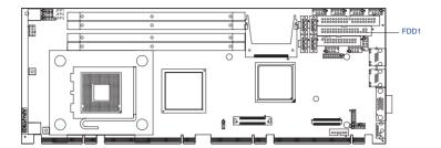
You can attach up to two floppy disk drives to the PCE-5120's on board controller. You can use 3.5" (720 KB, 1.44 MB) drives.
