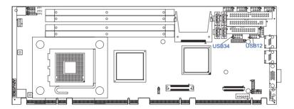
The PCE-5120 provides four on board USB 2.0 ports which support transmission rate up to 480 Mbps and is fuse-protected. To install the USB cable (p/n: 1700002314) bracket, find an empty slot in your chassis and unscrew the plate that covers the end of the slot. Screw in the bracket in place of the plate. Next, attach the USB connector to USB12 and USB34 on the CPU card.
