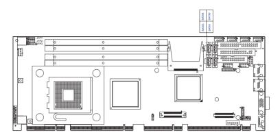
In addition to the EIDE interfaces (up to two devices), the PCE-5120 features a high performance serial ATA2 interface (up to 300MB/s) which eases cabling to hard drives with thin and long cables. These four port can be configured as RAID 0, 1, 5, 10 applications.
