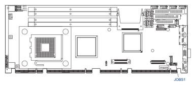
(JOBS1) is a 2-pin connector for setting enable/disable alarm while the On Board security event acts.
