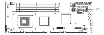
The parallel port is normally used to connect the single board computer to a printer. The PCE-5120 includes an onboard parallel port, accessed through a 26-pin flat-cable connector, LPT1. The card comes with an adapter cable which lets you use a traditional DB-25 connector. The cable has a 26-pin connector on one end and a DB-25 connector on the other, mounted on a retaining bracket. The bracket installs at the end of an empty slot in your chassis, giving you access to the connector.
