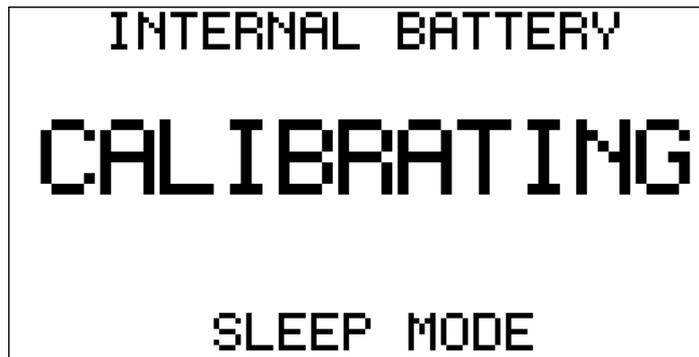
After the device recalibrates the internal battery charge reference level, it will automatically restart and you should see the Battery icon (on Spectrum Analyzer screen) showing full charge.
