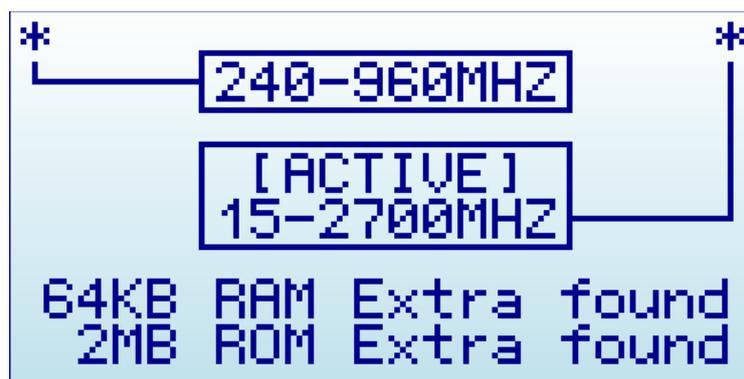
**Important:** Only one of the two SMA connectors is enabled at any given time. You select the active one using the Module option in the Frequency Menu, see page 14.
