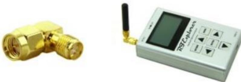
This RF connector is ideal to use RF Explorer deployed horizontally, with any antenna connected onto it.
