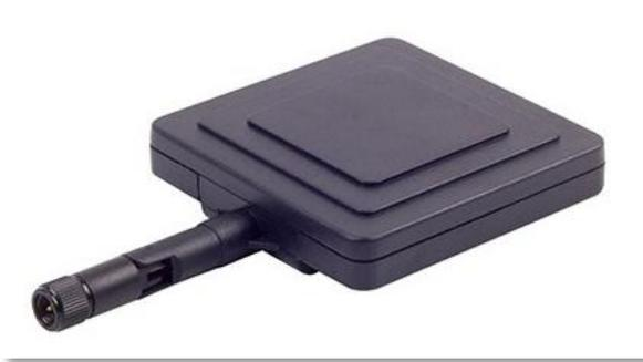
The directional patch antenna is a high gain, excellent choice to use RF Explorer analyzer to scan in a specific direction. As opposed to omnidirectional antennas such as dipole type, this patch antenna has an 8dBi gain in the front face. It includes a true SMA connector (not RP-SMA as most in the market) and therefore fits perfectly in all RF Explorer models.
