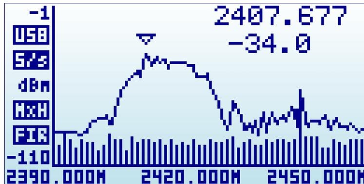
The X axis represents frequency in MHz and Y axis display actual received power in dBm or dBuV (selectable). In this example above, the frequency span goes from 2390 MHz to 2450 MHz (that is a 60MHz range), and the visual amplitude goes from -1 dBm to -110 dBm.
