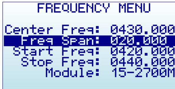
Selecting a span of 10MHz, the Start/Stop frequency changes accordingly:
